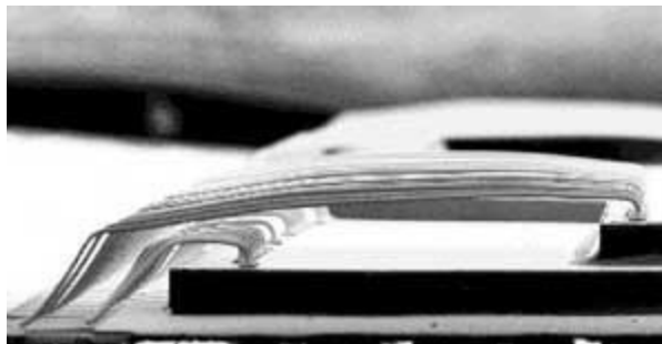
Figure 5. Forward ball bonding loops in stacked die applications.
